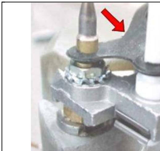
12. Detail of the cup gasket which has replaced the o-ring.
