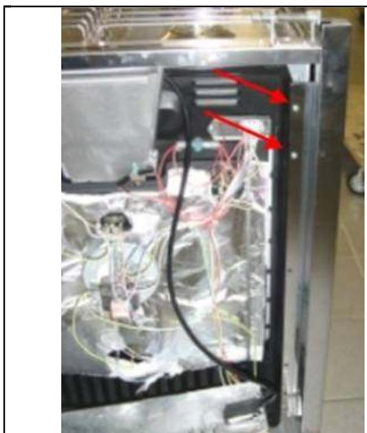
7. ...and remove the screws fixing the back side of the appliance.
