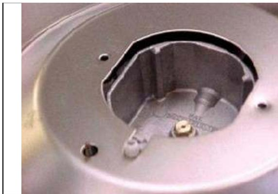
11. Positioning of the cup, such to let the replacement of the thermocouple/igniter plug, without further forcing the inflexion of the Bundy tube.
