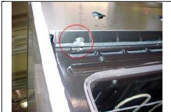
3. Unscrew the three screws (the others are at the center and on the right), that fix the front panel to the front panel head section, put it in the lower edge of the component.
