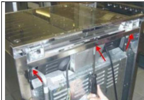
2. Remove the fixing screws for the splash board and then take out the part.
